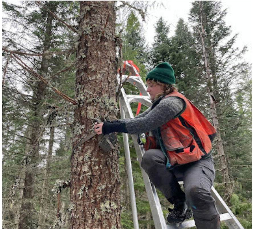
(Right) NNRG Forest Technician Nora Halbert installs a camera and a stadia rod to measure the accumulation and ablation of snow. Photo Credit: Jaal Mann/NNRG
